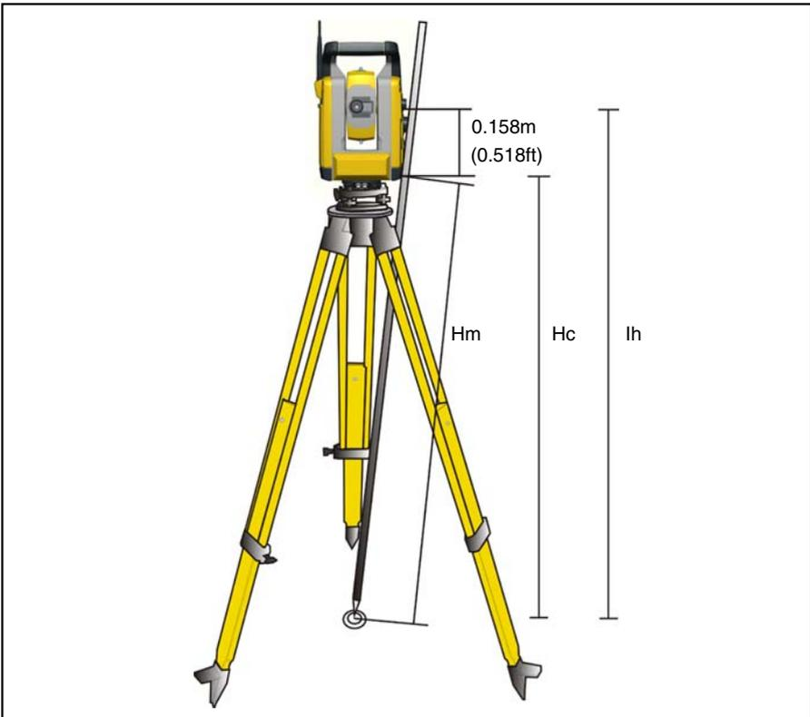
Figure 4.24 Instrument height measurement
