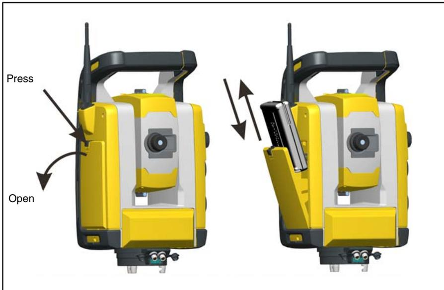
Figure 3.12 Removing and replacing the internal battery
