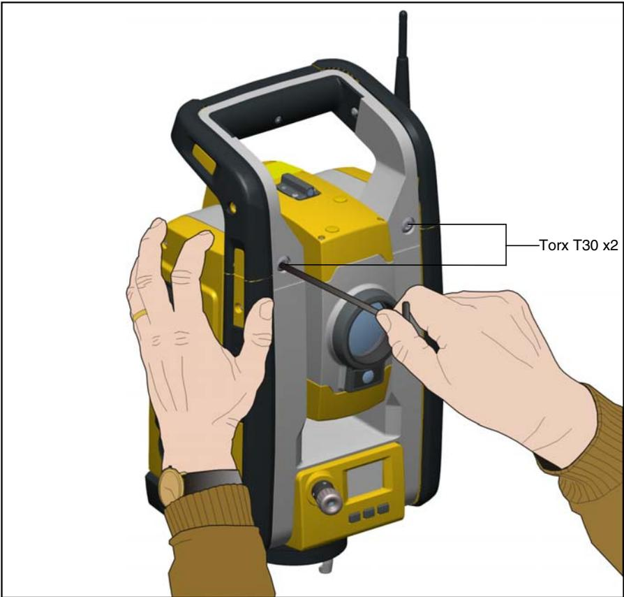
Figure 5.40 Removing the Trimble SPSx20 Total Station handle
