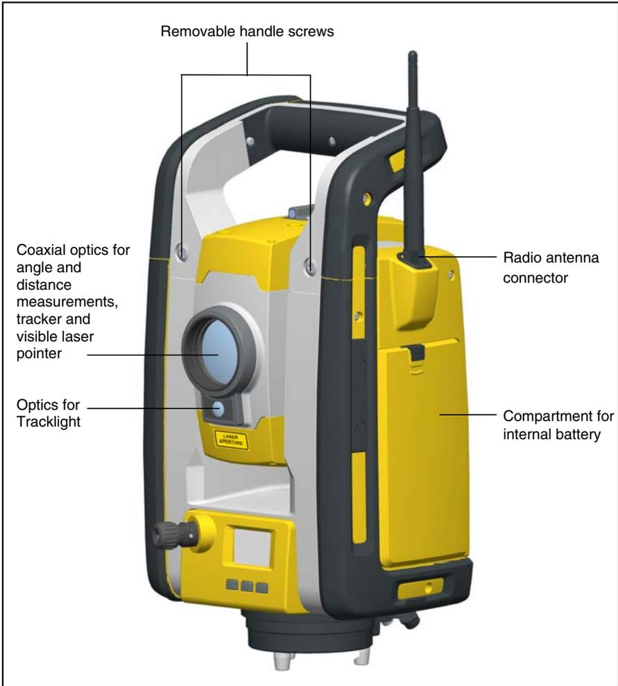
Figure 3.8 Front view of the Trimble SPSx20 Total Station
